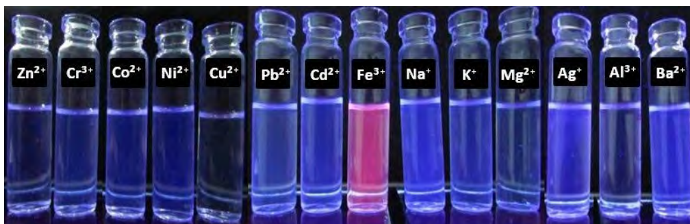
Figure 3.7 The photographic image of metal ions (20 \mu\text{M} ) solutions with ligand (PYAP, 10 \mu\text{M} ) under UV light illumination
